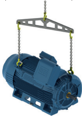
Figure 7 - Lifting with vertical chains.
